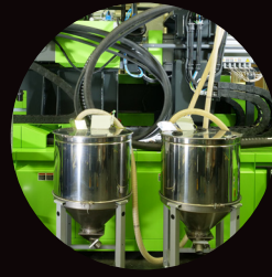
Virgin resin and PCR coinject into Regensis machine
